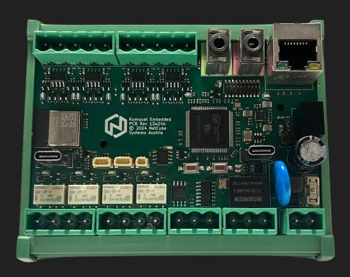
The Kumquat is a compact and versatile embedded system powered by the Allwinner V3s SoC. It offers robust connectivity options, extensive I/O capabilities, and support for popular programming languages. With its powerful features and flexible design, the Kumquat is ideal for a wide range of industrial, IoT, and embedded systems applications.
