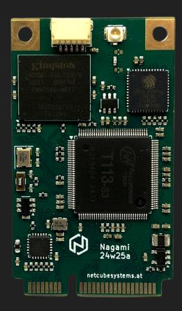
The Nagami is a compact and powerful embedded module built around the Allwinner T113-s3 SoC. With dual ARM Cortex-A7 cores, integrated HiFi4 DSP, built-in storage, and rich peripheral options, the Nagami delivers high performance and flexibility in a familiar miniPCIe full-size form factor. It's a perfect fit for demanding industrial, IoT, and embedded applications.
